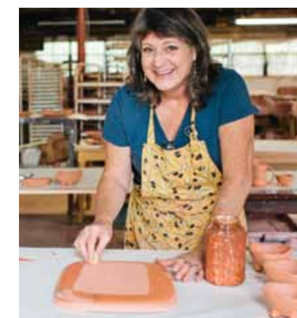
Before glazing the bisque-fired pieces, Tena applies a layer of wax to the bottom of each piece.
